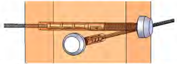
Figure C. For corners, offset your holes by 1/2" to avoid stud interference and/or weakening of posts.
