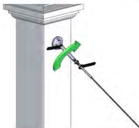
Figure R. Hold the swage terminal still with 3/16" wrench and using a 5/16" open wrench, rotate tensioner body to tension.
