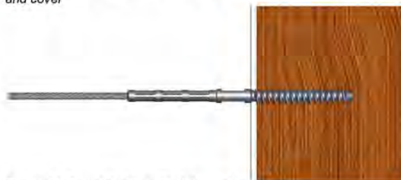
Figure N. Completed Lag Stud Assembly
