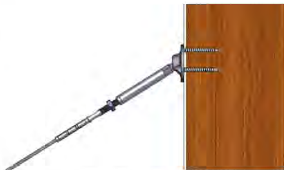
Figure Q. Extend the stud leaving 3/4" of thread for 20' or less. For every additional 10', leave another 1/4" of thread exposed.
