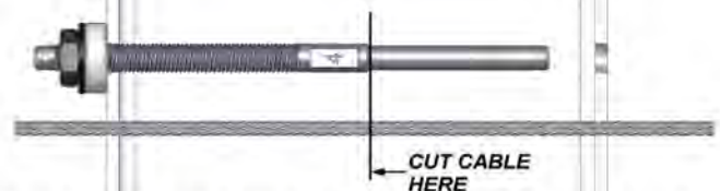
Figure F. Pull the cable tight to the back of the swage fitting. Mark and cut the cable there and swage the second fitting in accordance with swaging tool instructions
