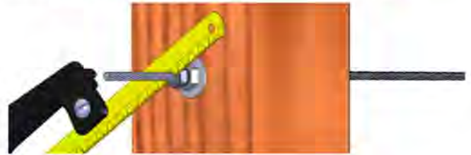
Figure I. Trim excess cable with a hack saw or grinding disk in order to attach the cap for a finished look.
