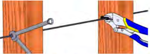
Figure H. Use a cable grip pad with vice grips to hold the cable tight.
