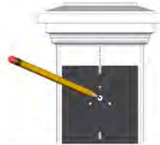
Figure B. Atlantis offers a template to help you find your centers.
