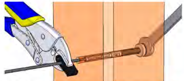
Figure K. METHOD 2: Using a HandiSwage Cable Grip Pad and vice grips, hold the cable in a fixed position while tightening the tension nut.
