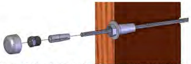
Figure G. Put the cable through the flush fitting. Push it against the back of the post and put the cable tight.
