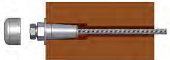
Figure D. Re-drill the back end of the post with a 7/16" bit to accept the flush fitting.
